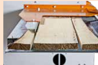
The board is edged in a quick and controlled operation.
