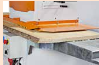
The side cover is opened by the workpiece when you are edging extra wide boards.
