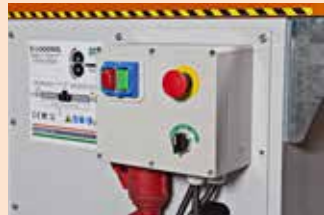
You operate the three motors of the machine from the control panel.
